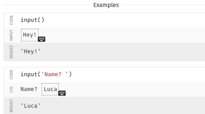
Figure 9.11. Examples in Judicious for Python's input function, showing separately the output (I/O) and the result of the evaluation.
